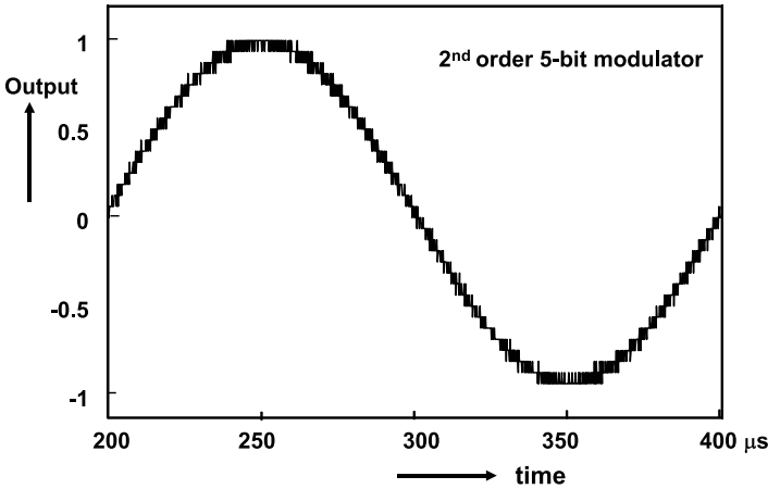
Fig. 9.38 The reconstructed output wave form of a 5-bit quantizer in a sigma-delta modulator
